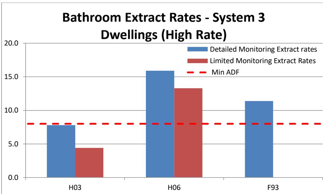
9.21 Low rate (trickle speed) extract ventilation rates were measured in all three System 3 homes. The assumption, as per measurements taken during the walkthrough survey, is that the fans in each home are typically used at trickle speed (boost being selected only when bathroom light is on or by occupant use of boost switch in kitchens). The combined total fan
